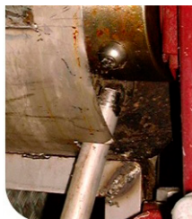
Magnetic trigger sensor for roll/shaft rotational speed measurement
