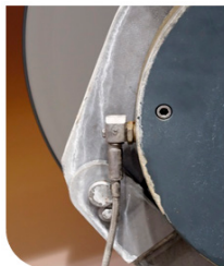
Vibration sensor for wet and humid environment
