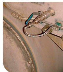
Pressure sensor for dynamic pulsation measurement in short circulation and head box
