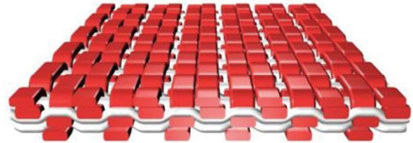
Figure 18. TamStar HighSpeed groove structure improves high pressure cleaning.
