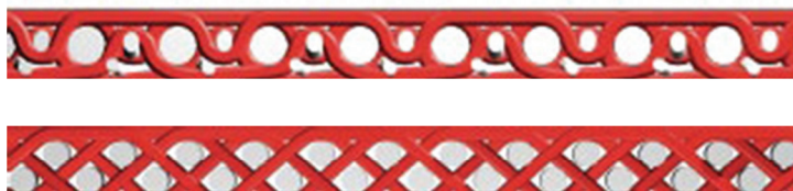
Figure 10. The double-cloth structure ensures better wear potential.
