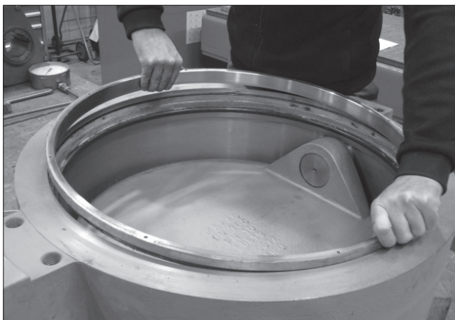
Fig. 40 Taking out the seal ring
