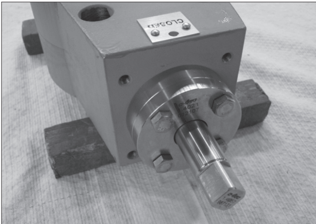
Fig. 53 4 bolts on the actuator side
