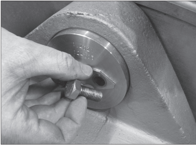
Fig. 44 Removing the clamping plate
