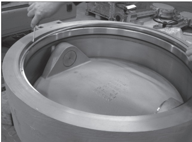
Fig. 39 Taking out the retainer ring
