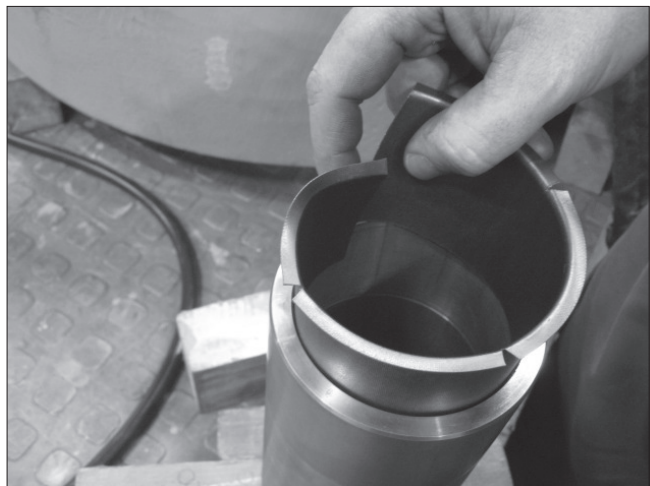
Fig. 49 Replacing the Metaloplast bearing
