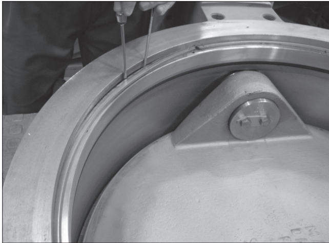
Fig. 38 Lifting the retainer ring
