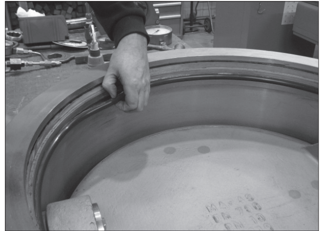
Fig. 41 Taking out the seal ring
