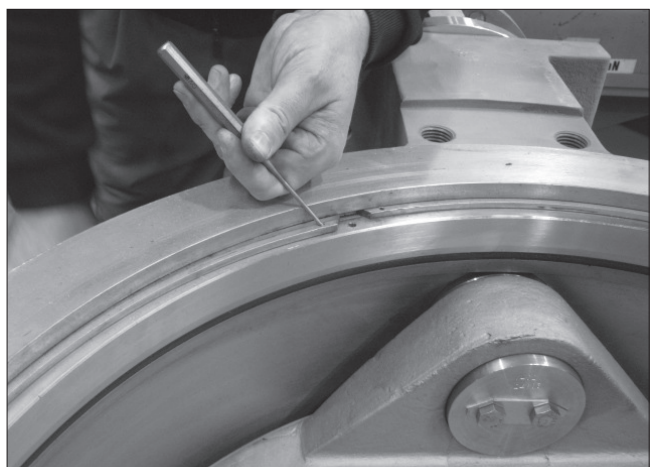
Fig. 37 Releasing the retainer ring using a drift punch
