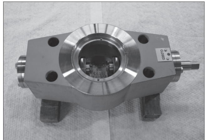
Fig. 52 Disc in 180°-position
