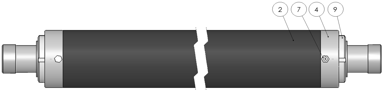
Figure 16. Installing the cover hose.
