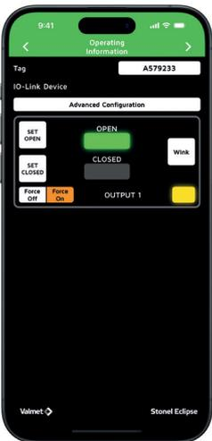
Customize the tag for a device, change the address, force the solenoids on or off, wink the device, and set the valve limits.
