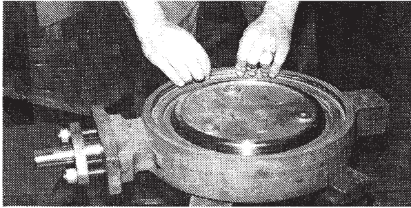
Placing Spring Into Groove
